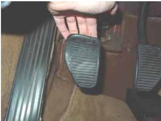
3. Clean the front surface of the factory clutch/brake pedal sheet metal using degreaser and a shop towel or rag.
